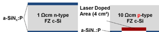
Figure 3: Left: Structure used to extract lifetime and SRV Right: Structure used to measure R_{sheet} and doping profile.
